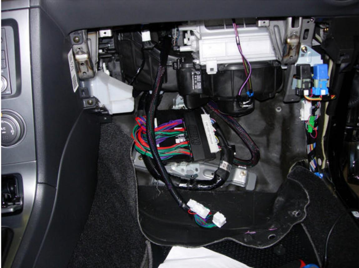
3. Route the long side of the harness up behind the glove box as seen in the picture above.
