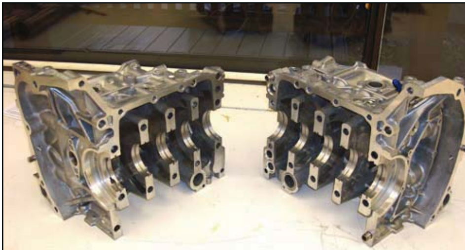
THE SUBARU EJ25 ENGINE BLOCK IS BEEFY. MPS USES ONLY THE FINEST INGREDIENTS, LIKE THE BLOCK INTENDED FOR SUBARU'S TURBOCHARGED APPLICATIONS.
