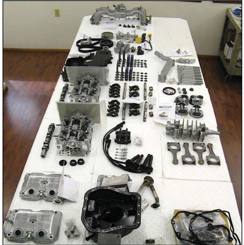
THE EJ25 ENGINES ARE TORN DOWN AT MPS TO BE BLUEPRINTED AS PART OF AIRCRAFT-SPECIFIC MODIFICATIONS. THESE ARE IMPORTANT FOR LONGEVITY.
